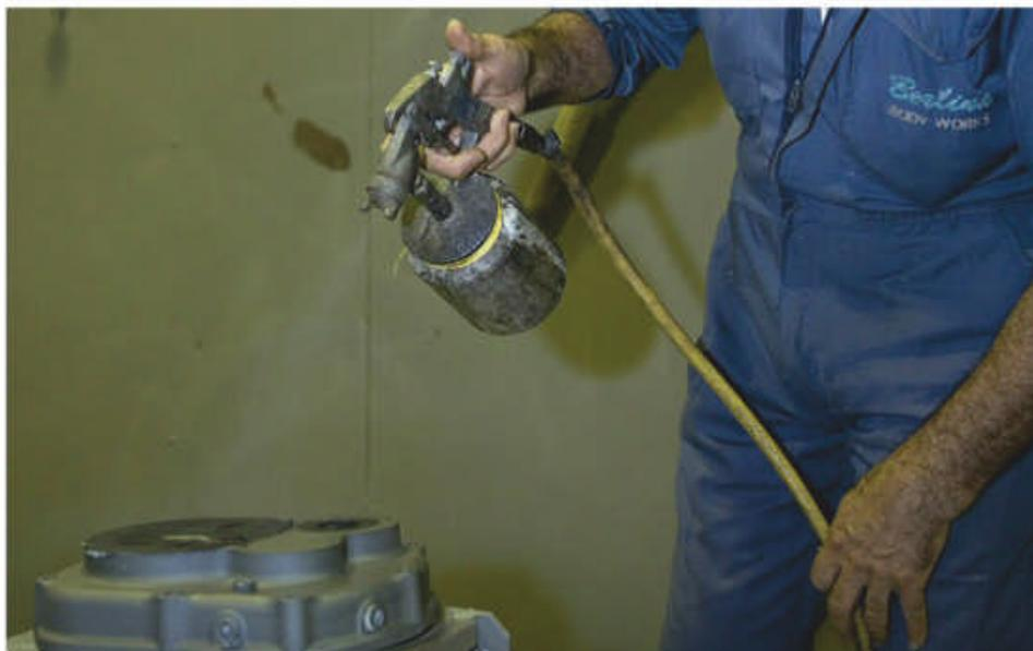
▲ **STEP 9** Most parts are finished with a metal prep coat to prevent stripped surfaces from rusting.
