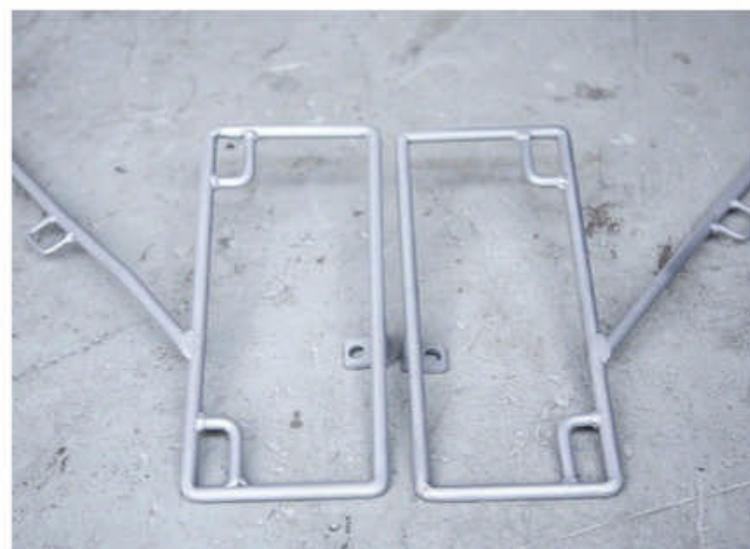
◀ **STEP 10** These stripped pannier rails won't be prepped as they're heading out to be powder coated; the prep coat would interfere with that process.
