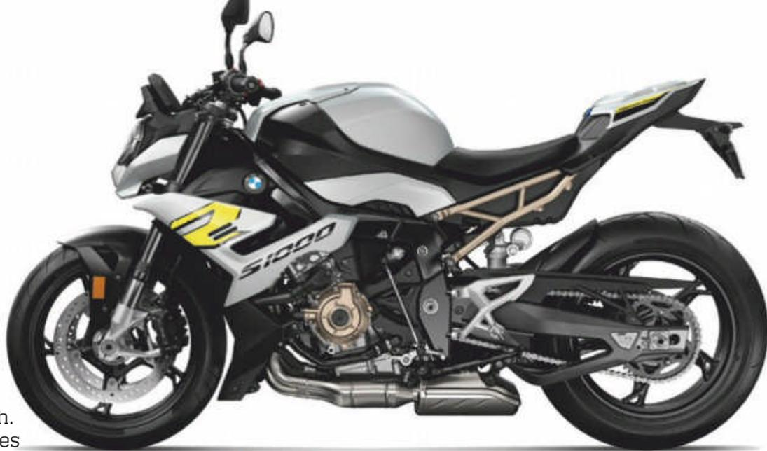
while the new beam frame contributes to an overall 6.5kg reduction in the bike's weight despite the extra components required to meet Euro5 regs. BMW claims a 0-200km/h time of 8secs flat, five percent faster than before.
