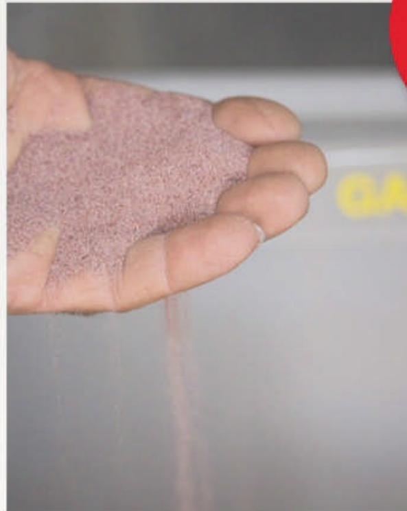
◀ **STEP 6** Garnet – basically machined-down granite – is also used for blasting. It's harder than plastic beads, and applied at a slightly higher pressure.
