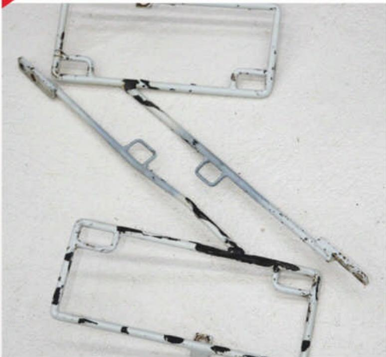
▲ **STEP 1** Parts like this need to be stripped of all old paint and surface rust before being refinished with paint or other coatings.
