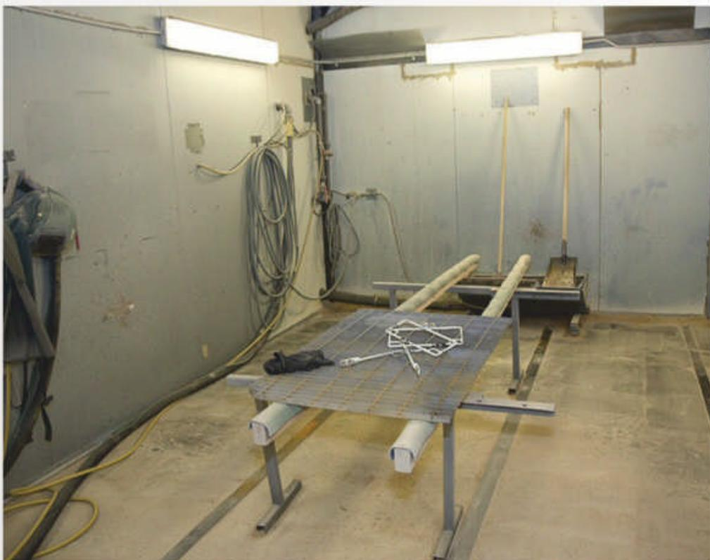
▲ **STEP 3** The part is placed in a sealed blasting room. The process is dry and environmentally friendly (all residue is bagged and recycled).
