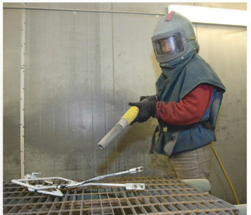
▲ **STEP 4** The plastic media is applied to the surface at about 15 psi. Although making short work of old paint and other materials, the relatively low pressure and lack of heat buildup ensures construction materials such as carbon fibre and plastic motorcycle panels can be stripped with confidence.
