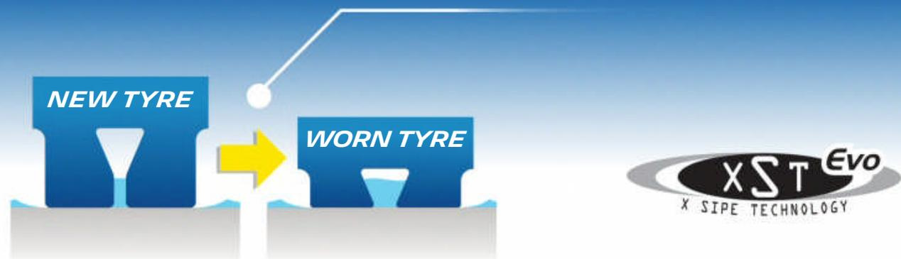
Over the kilometres, normal tread wear reveals ever wider grooves to increase the tyre's sea-to-land ratio and thereby maintain its ability to clear water.
