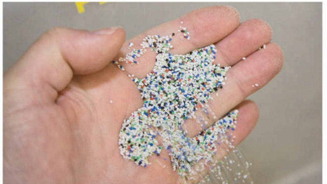
▲ **STEP 2** Plastic media consists of small plastic beads applied at force to the surface to be stripped. They are softer than most other compounds used in blasting and are applied at a much lower pressure. As a result, they don't cause panel buckling or other damage sometimes associated with other stripping methods.
